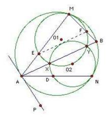
Let  $C_1$  and  $C_2$  meet at X and Y, and let AN meet  $C_2$  again at D. Then  $AE \cdot AM = AX \cdot AY = AD \cdot AN$ , so triangles AED and ANM are similar. Hence  $\angle ADE = \angle AMN$ .
