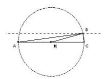
Area = AB·BC/2 (because  $\angle$  ABC = 90° = BM<sup>2</sup>/2 (required) = AC<sup>2</sup>/8 (because BM = AM = MC), so B lies a distance AC/4 from AC. Take B as the intersection of a circle diameter AC with a line parallel to AC distance AC/4.
