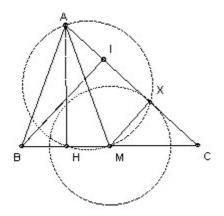
Let M be the midpoint of BC, AH the altitude from A, and BI the altitude from B. Start by constructing AHM. Take X on the circle diameter AM with MX = BI/2. Let the lines AX, HM meet at C and take B so that BM = MC. [This works because CMX and CBI are similar with MX = BI/2 and hence CM = CB/2.]
