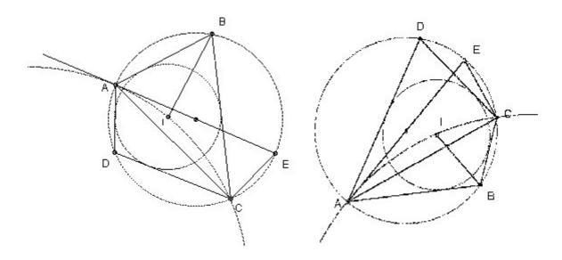
I be the center of the inscribed circle. Consider the quadrilateral ABCI.  $\angle$  BAI = 1/2  $\angle$  BAD and  $\angle$  BCI = 1/2  $\angle$  BCD, so  $\angle$  BAI +  $\angle$  BCI = 90°, since ABCD is cyclic. Hence  $\angle$  AIC = 270° -  $\angle$  ABC. So if we draw a circle through A and C such that for X points on the arc AC  $\angle$  AXC =
