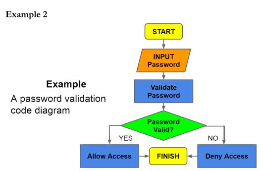
This is an example of a branching diagram. The branch occurs at the green diagram, the 2 paths are represented by the "yes" and "no" arrows. Notice that both path lead to the finish.
