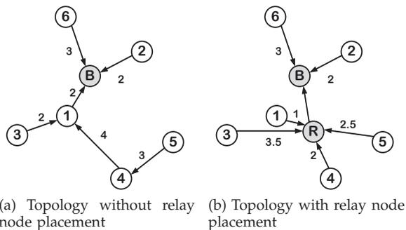
Fig. 3: Network topology with or without relay node placement. For (a), the energy cost is  $4^2 \times 2 = 32$ , which occurs at  $s_4$ . For (b), the energy cost is  $3.5^2 \times 1 = 12.25$ , which occurs at  $s_3$ .
